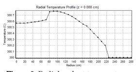
Figure 8. Radial coolant temperature distribution (*Prenpac*)
