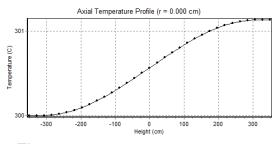
Figure 7. Axial coolant temperature distribution
