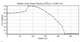
Figure 6. Linear power density in radial
