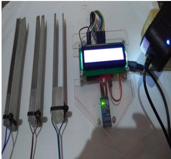
Figure 1. Measuring Water Content in Soil-Based Capacitive (AUKAK)
