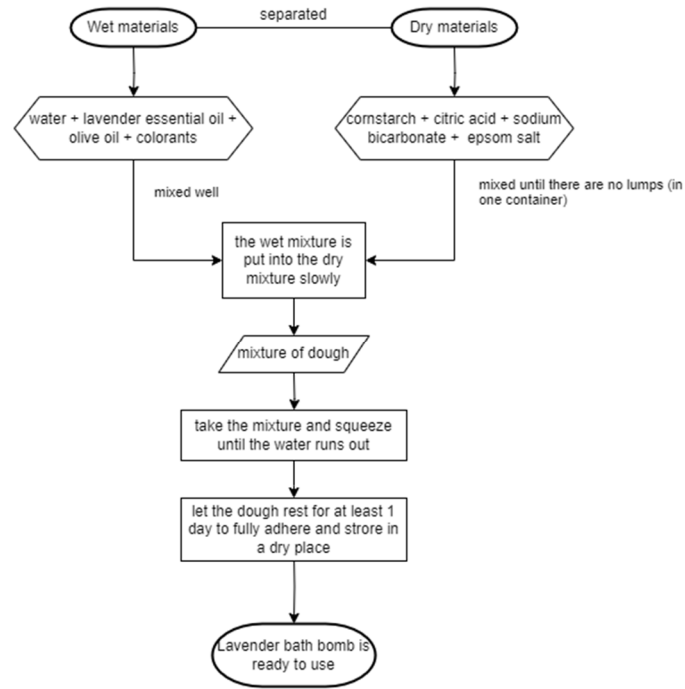
Figure 2. Schematic diagram of lavender bath bomb production
