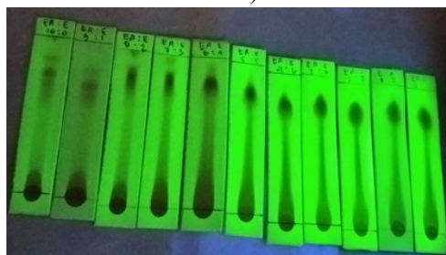
Figure 2. Preliminary KLT Results of Concentrated Extract of Parasite Coffee Flower ( Loranthus ferrugineus Roxb.) with Ethyl Acetate : Ethanol (10:0; 9:1; 8:2; 7:3; 6:4; 5:5; 4:6; 3:7; 2:8; 1:9 and 0:10)
