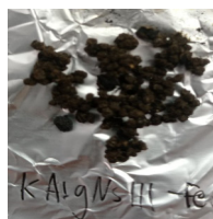
Figure 2. Activated Carbon/ Alginate/ Nanocellulose-Fe Composite Beads
