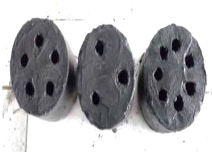
Figure 4. Catalytic converter with variations in the number of holes 3, 5 and 7
