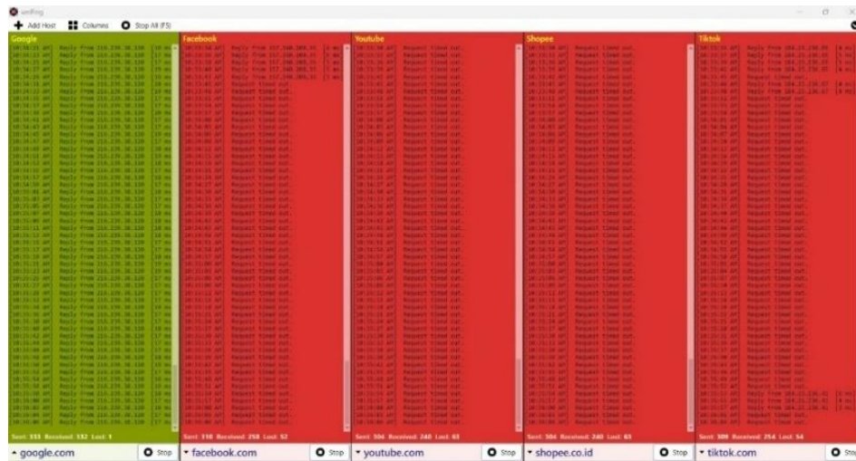
Gambar 7. Monitoring vmPing sesudah penerapan Firewall
