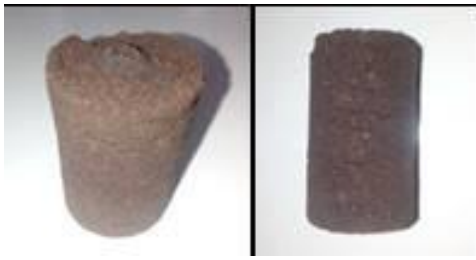
Figure 2. Briquettes at 150°C with 10% Binder Meanwhile, at a temperature of 250°C, the charcoal particles obtained from the briquettes with 10% tapioca binder appeared to be unevenly mixed, exhibiting a smooth texture with slight cracks, making the briquettes prone to breaking and resulting in a dark brown color, as shown in Figure 3.
