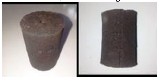
Figure 3. Briquettes at 250°C with 10% Binder
