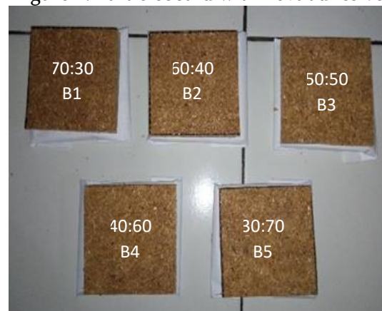
Figure 3. Particleboard with 15% adhesive
