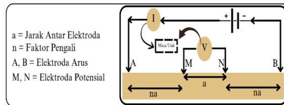
Figure 2. Schlumberger Configuration Geoelectric Method
