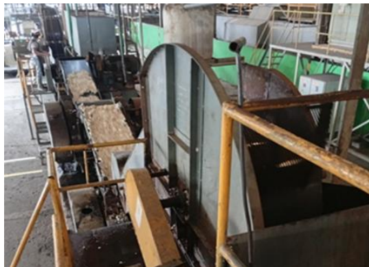
Figure 4. Creping Process on a Crepe Machine
