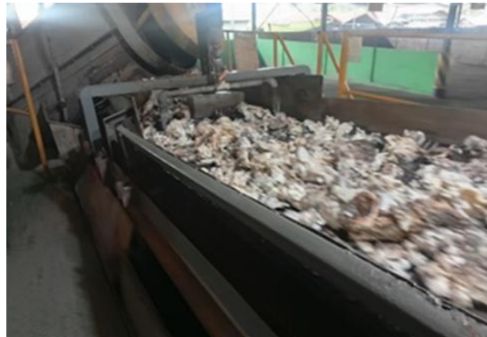
Figure 3. Shredding and Cleaning of Raw Rubber Material Process
