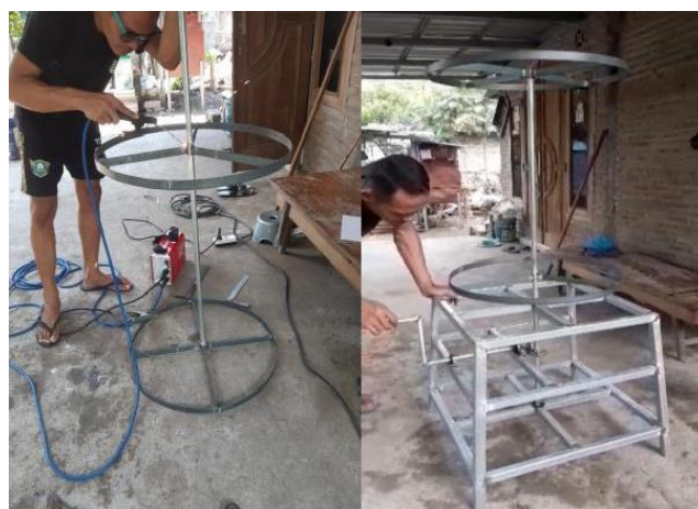
Figure 10. Welding process of iron plate, iron pipe and wheel gear assembly and lacker (Source: Ratih, 2024)
