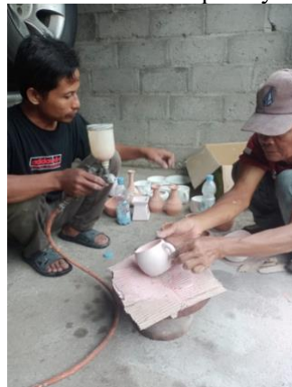
Figure 4. Glaze Application Process Using Spray Technique Source: (Suharson, 2025)
