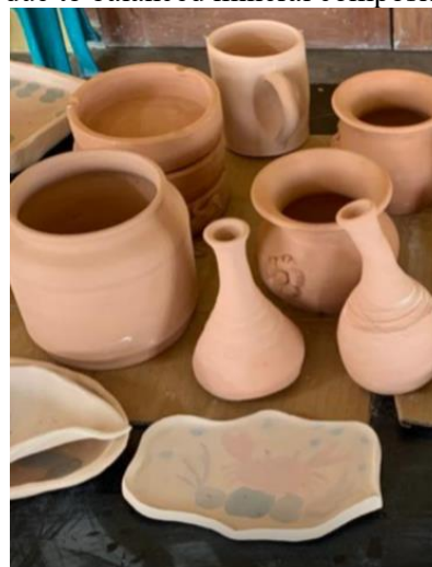
Figure 2. Bisque Firing Result Source: (Suharson, 2025)
