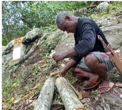
Gambar 4. Proses Penandaan Lubang Resonansi Bunyi Sumber: Peneliti, April 2024
