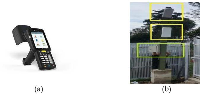
Gambar 4. (a) Hand Handheld RFID, (b) RFID Gate
