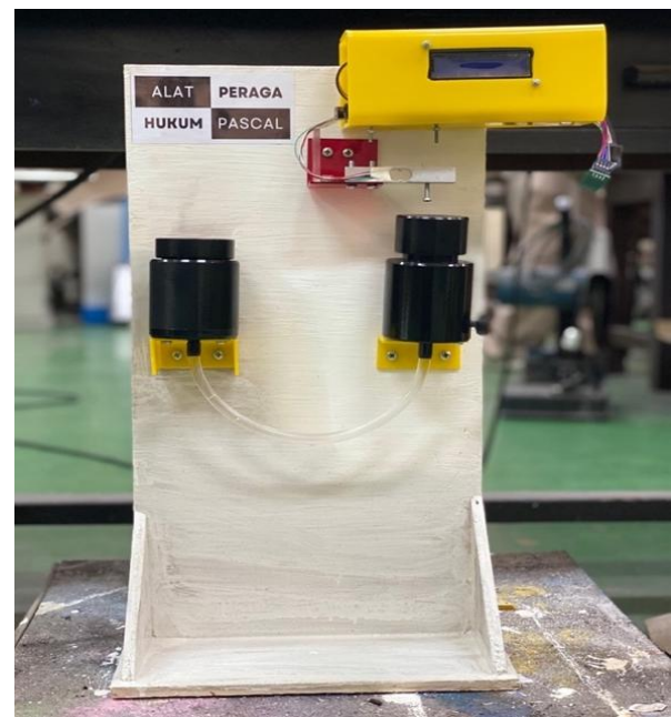
Figure 3. Visualization of the Final Product of Pascal Law Learning Media Based on Arduino Uno
