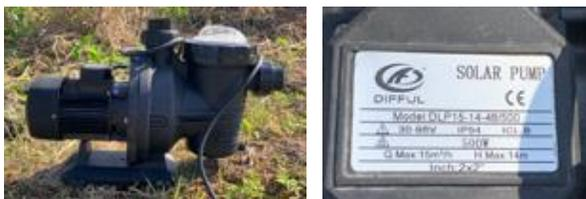
Gambar 6. Solar pump 500 Watt
