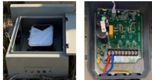
Gambar 8. Box Controller dan controller
