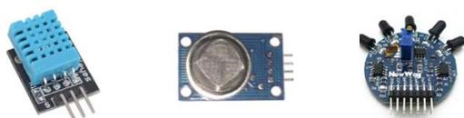
(a) Sensor suhu DHT 11      (b) Sensor asap MQ-135      (c) Sensor api channel
