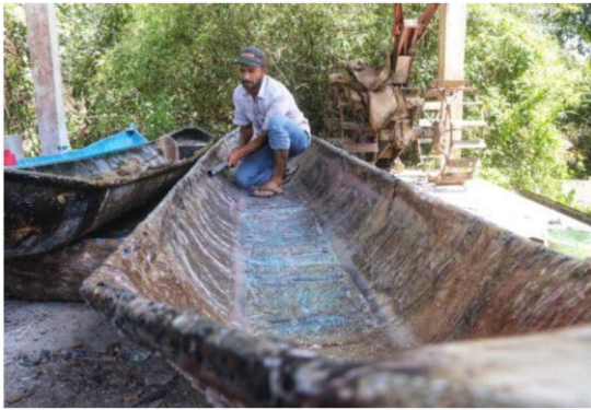
Gambar 7. Proses perapian permukaan perahu sampan hybrid fiberglass-goni bekas
