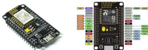
Gambar 1. (a) NodeMCU ESP8266 v5, dan (b) Pin Out NodeMCU ESP8266 v5
