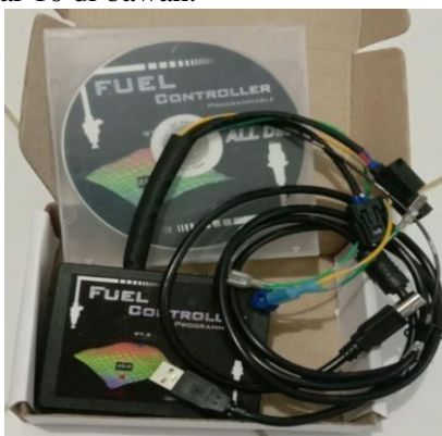
Gambar 11. ECU STANDALONE BERBASIS ATMEGA 2560
