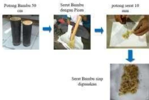
**Gambar 8.** Proses Persiapan Serat Bambu
