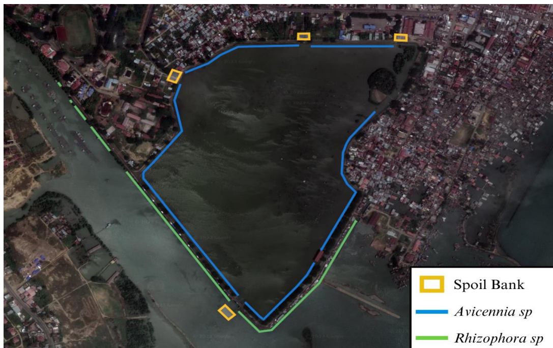
Fig 2. Management map of sediment traps and vegetative systems of the Pusong reservoir in Lhokseumawe City
